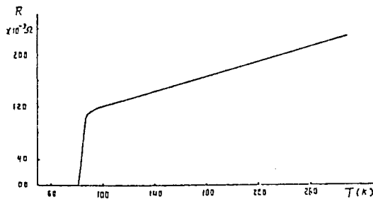
Fig.2 Temperature dependence of resistance for Y-Ba-Cu-O thin film
