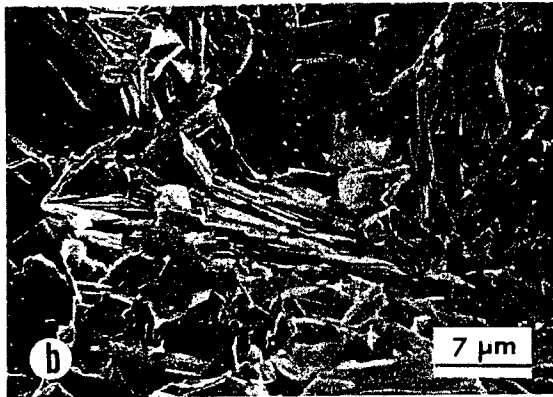
Fig.5 SEM images showing the stages of crystal growth from the 30 to 37 A phases. The specimens were heated finally at 870°C for 12 hr (a) and at 875°C for 12 hr (b).
