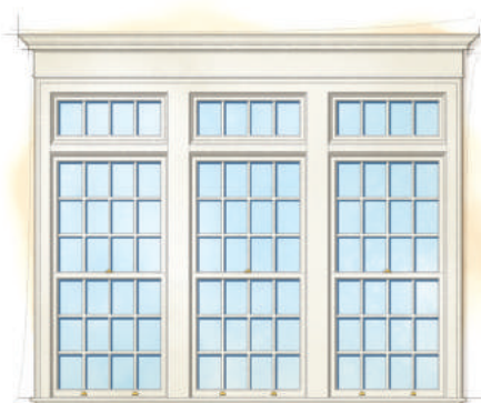
Double-hung and transom window combination (interior)
