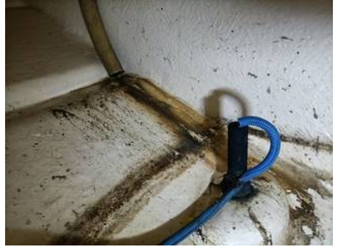
Figura 5: central bilge some dirty from grey tank
