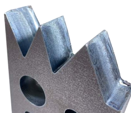
12kW Fiber Laser cutting machine Material: SN490C Thickness 25mm
