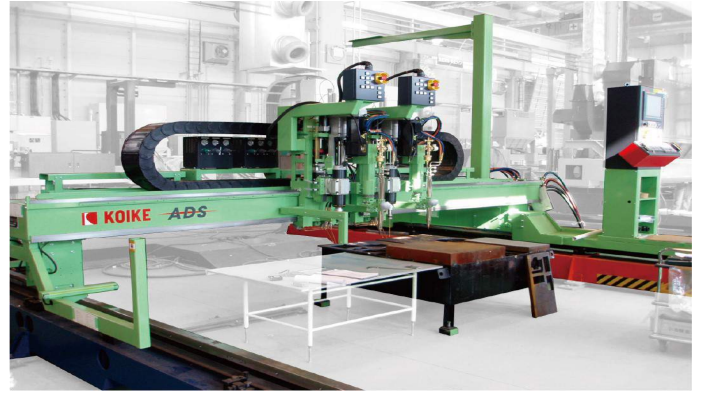
CNC Piercing hole drill specialized machine specialized in piercing holes where cutting is necessary.
