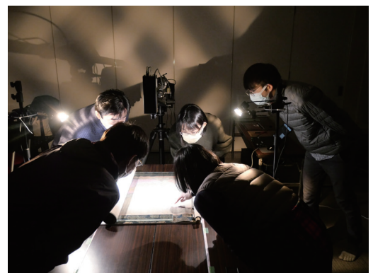
Examination of painting materials using a hyperspectral camera (Tokyo National Research Institute for Cultural Properties)
