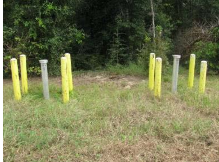
Photo 152: Monitoring well pairs located near wooded area east of Process Sedimentation Pond.
