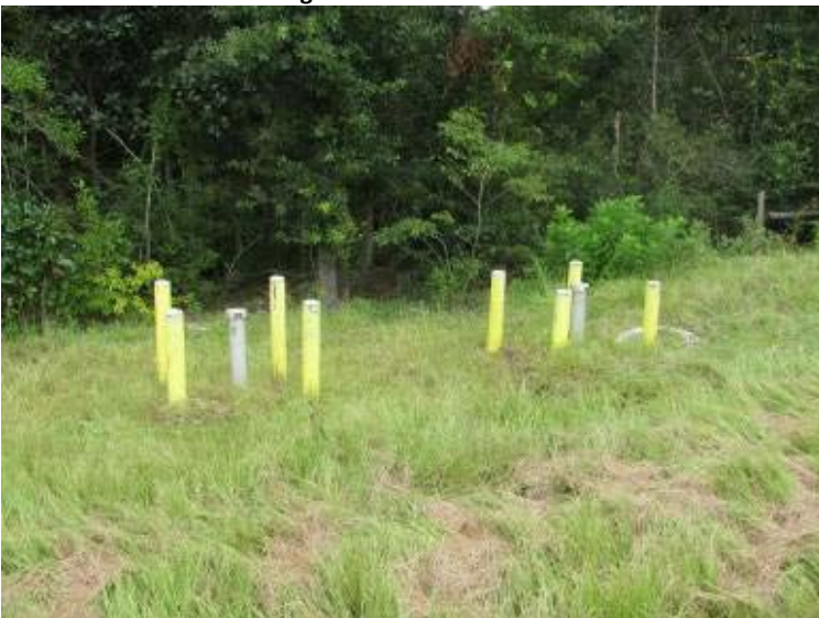
Photo 139: Groundwater monitoring wells located beyond toe of slope of north embankment of Process Sedimentation Pond looking north.
